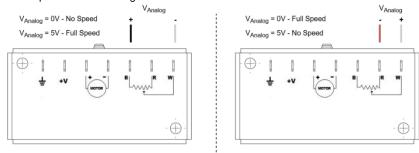
CAUTION: When using an analog command option, note that any improper connection may result in motor runaway or no motion control. Be sure not to exceed 5V input or damage to the control can result.
